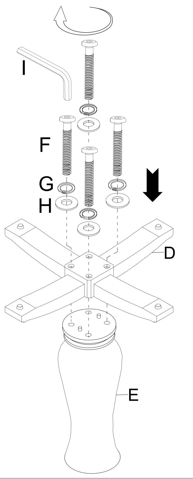
2 Attach Table Top Cross Base (B) to Pedestal Column (E) using Bolt (F), Spring Washer (G) and Flat Washer (H) with Allen Wrench (I).
