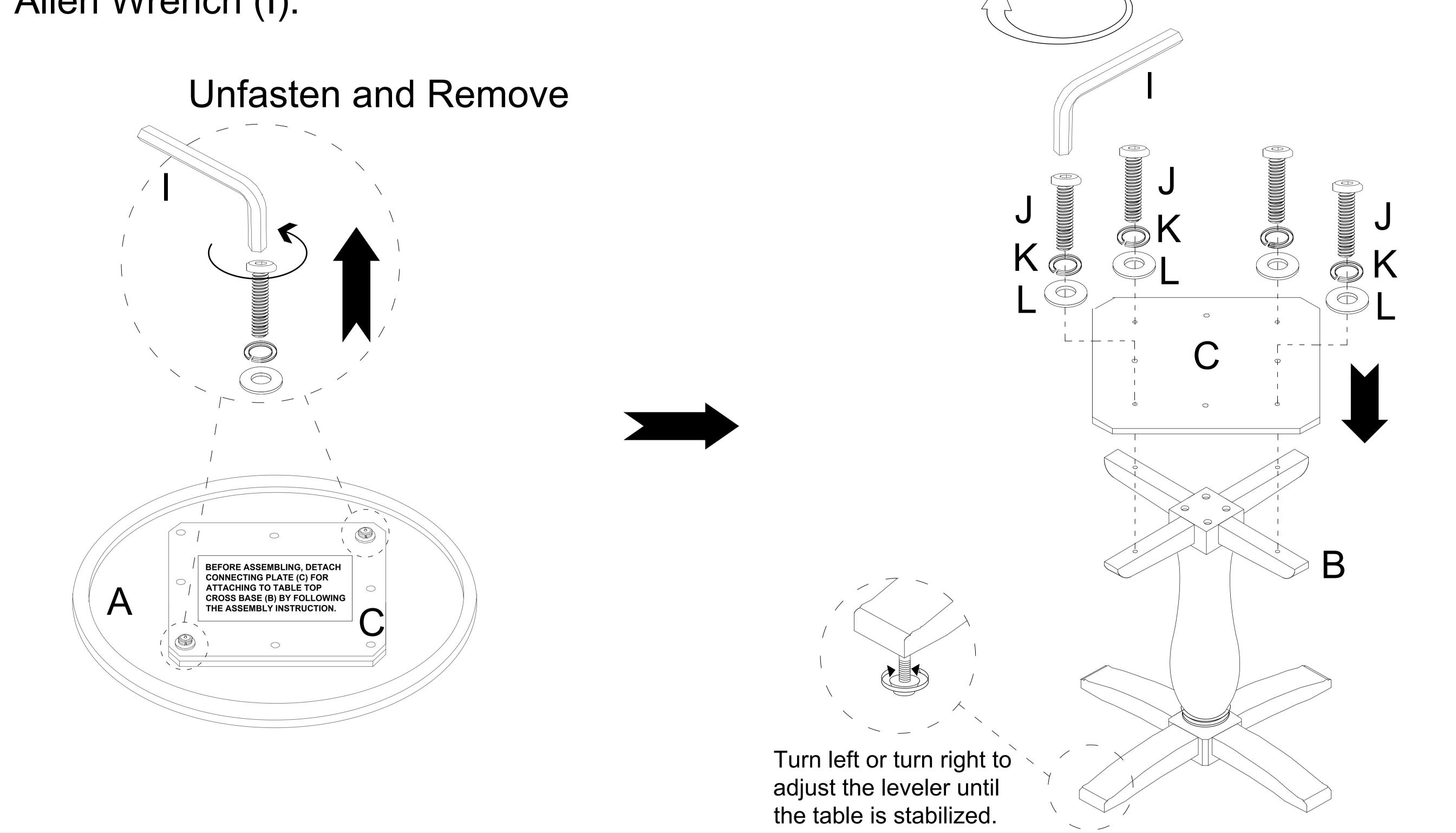
Attach Connecting Plate (C) to Table Top (A) using Bolt (J), Spring Washer (K) and Flat Washer (L) with Allen Wrench (I).
