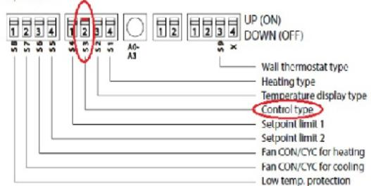
S3 must be on for wall thermostat control. Cycle the PTAC unit power off and on after making the change, for the selection to take effect.
