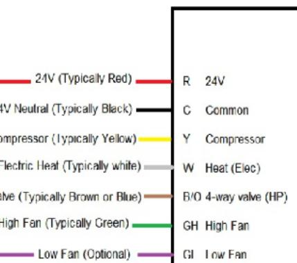
The S3 dip switch must be turned on and the S9 dip switch must be turned off. Also, please note that some wired controllers need to be programmed for switching the 4-way valve internally. Please read the wired thermostat directions to verify if this is required on you t-stat.
