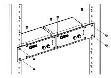
TSD-RRMK Optional Rear Rack Mounting Kit - For complete flexibility in mounting a TSD or TSD external power supplies the optional TSD-RRMK is available. The TSD-RRMK can support mounting of either two larger TSDs with external power supplies or up to 4 TSD models. **Note:** Only use the included M3 x 4mm screws as other screws may be too long and will cause internal damage to the TSD.
