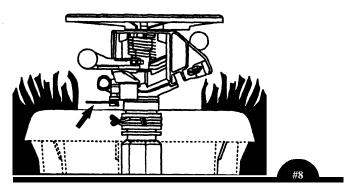
NOTE: You will need to fine-tune the arc with the pattern adjusters while the sprinkler is operating.
