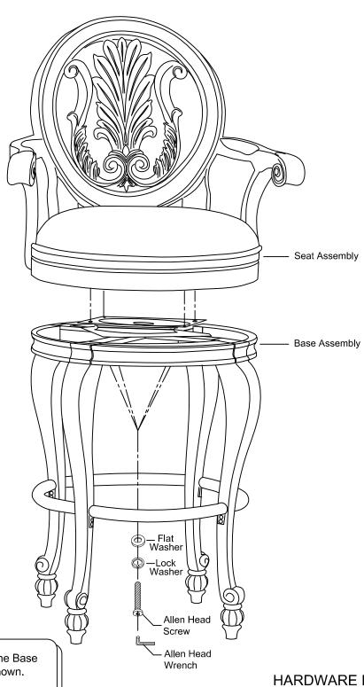
Attach the Seat Assembly to the Base Assembly with hardware as shown.
