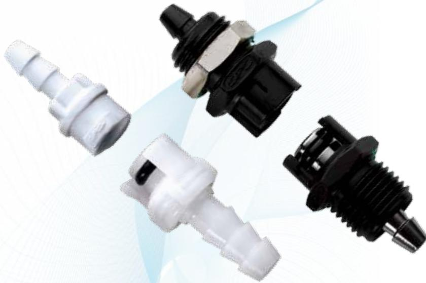
The **SMC** and **SMF1** are among CPC's smallest couplings. These twist-to-connect couplings provide a reliable and more secure alternative to luer-type connections. They also allow for the tubing to rotate freely when connected. This important feature prevents both kinked tubing and accidental disconnection during use. The SMC Series is also available with optional RFID (Radio Frequency Identification) capability (page 98) and in polycarbonate material (page 102).
