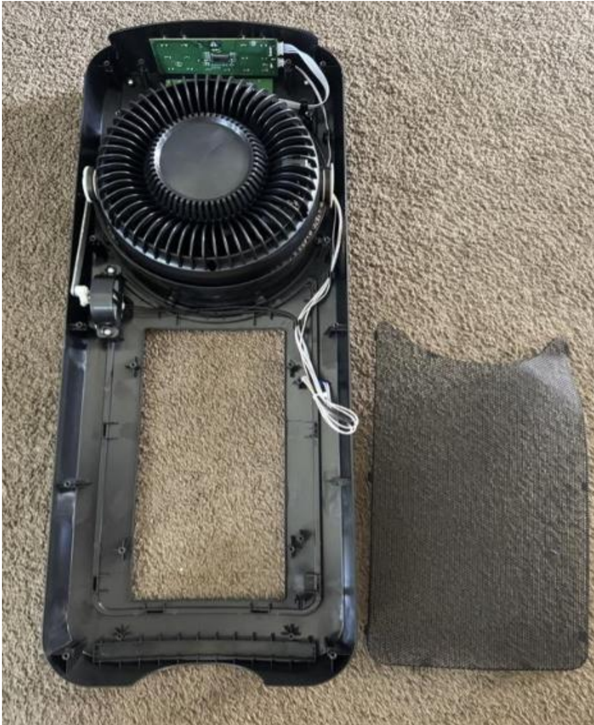
Photo 4 - Fan Assembly View
