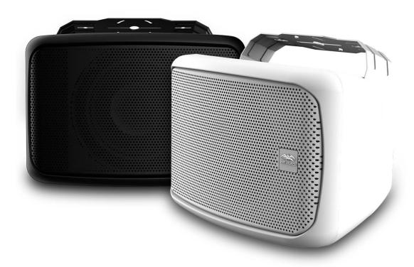
The VS-8 PRO utilizes Wet Sounds' Horn Loaded Compression Driver (HLCD) technology, combined with a reinforced composite mid-bass driver, and features  $4\Omega$  and 70v adjustable tap settings, including 40W, 80W, 120W & 160W. The VS-8 PRO provides a balanced sound for large, open-air environments. The weatherproof enclosure features Wet Sounds' reaction technology, consisting of opposing dual aluminum passive radiators to deliver superior bass response.
