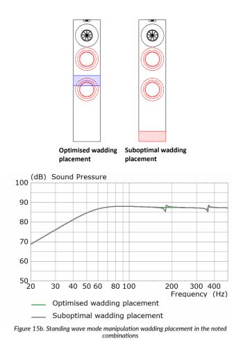
The new Q floorstanders employ a combination of the three approaches; mode cancellation, mode suppression and optimised attenuation; to minimise the occurrence and audibility of standing wave modes inside the cabinet. This is shown in Figure 16.
