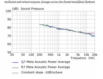
Figure 20. Q7 Meta and R7 Meta acoustic power averages
