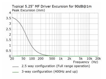
Figure 5. Typical excursion requirements for a 5.25" MF driver in a 2-way and 3way configuration. Passband level of 90dB at 1m
