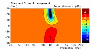
Figure 2. Schematic driver arrangements on an infinite baffle (top), summed on-axis response at 1m on tweeter axis (middle), normalised vertical directivity contour for both driver arrangements (bottom)
