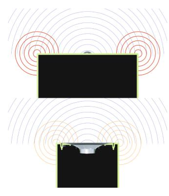
Figure 11. Diagrammatic representation of the tweeter in a flat baffle (top) and in the Uni-Q arrangement with a Shadow Flare (bottom). Direct sound is in blue, and secondary, diffracted sound (red and orange)
