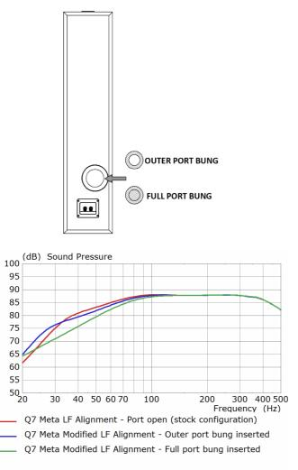
Figure 17. Adjustable port tunings for the Q7 Meta using the supplied two-part bung
