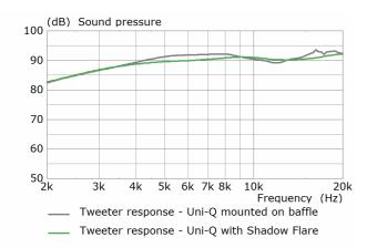
Figure 13. Tweeter response with (green) and without (grey) the Uni-Q Shadow Flare
