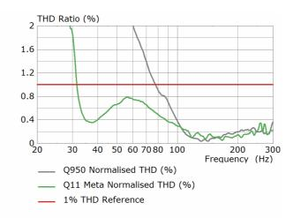
Figure 9. Q950 (grey) and Q11 Meta (green) low-frequency in-situ THD ratio (%) in response to 90dB SPL (fundamental). Also shown is the 1% THD threshold (red)
