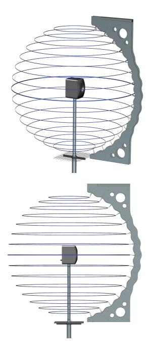
Figure 21. KEF's anechoic chamber microphone array used for the development of Q Series with MAT
