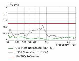
Figure 7. Q950 (grey) and Q11 Meta (green) midrange in-situ THD ratio (%) in response to 90dB SPL (fundamental). Also shown is the 1% THD threshold (red)
