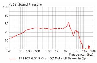
Figure 8. 6.5" 8 Ohm LF (Q7 Meta) 2pi infinite baffle response (2.83Vrms at 1m)
