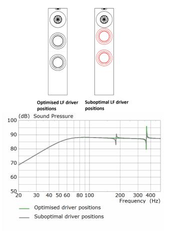
Figure 15a. Standing wave mode manipulation driver positions in the noted combinations
