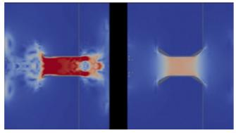
Figure 18. Computational Fluid Dynamics (CFD) model showing the effects of a straight tube (left) and one with optimised flared profiles at either end (right) on the turbulence behaviour,
