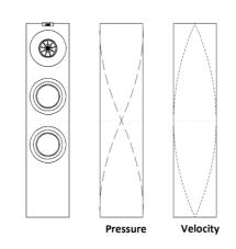
Figure 14. Standing wave pressure (middle) and velocity (right) mode shapes using Q7 Meta as example
