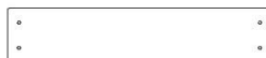
M20 PANNEAU MURAL - W4L14590 (x2) 5/8 po x 3 3/8 po x 16 1/4 po (16 x 86 x 412)
