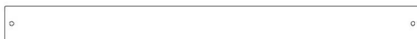
H8 SUPPORT DE PLANCHER - W4L22682 (x1) 1 po x 3 3/8 po x 40 3/8 po (24 x 86 x 1024)
