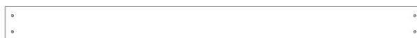
M19 PANNEAU MURAL - W4L14589 (x2) 5/8 po x 3 3/8 po x 40 5/8 po (16 x 86 x 1032)
