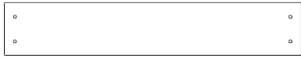
M102 | SUPPORT ARRIÈRE - W4L17614 (x1) | 5/8 po x 3 3/8 po x 19 1/8 po (16 x 86 x 486)
