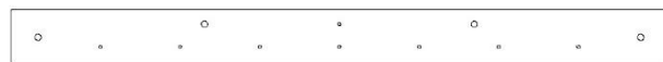
H2 SUPPORT DE PLANCHER - W4L22676 (x1) 1 po x 3 3/8 po x 40 3/8 po (24 x 86 x 1024)
