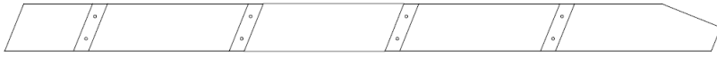
H75 | MONTANT DROIT - W4L17612 (x1) | 1 3/8 po x 3 3/8 po x 50 3/4 po (36 x 86 x 1290)
