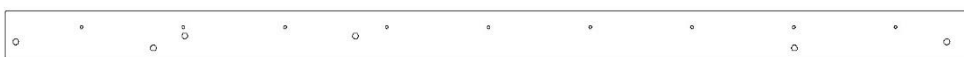
H5 SUPPORT DE PLANCHER - W4L22679 (x1) 1 po x 3 3/8 po x 64 3/4 po (24 x 86 x 1644)
