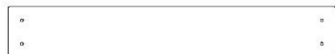
M13 PANNEAU MURAL - W4L14583 (x9) 5/8 po x 3 3/8 po x 22 po (16 x 86 x 558)
