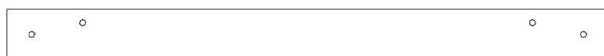
H6 SUPPORT DE PLANCHER - W4L22680 (x1) 1 po x 3 3/8 po x 40 3/8 po (24 x 86 x 1024)
