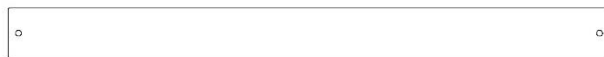
M2 SUPPORT DE PLANCHER - W4L14572 (x1) 5/8 po x 3 3/8 po x 40 3/8 po (16 x 86 x 1024)
