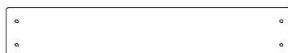
M102 SUPPORT ARRIÈRE - W4L17614 (x1) 5/8 po x 3 3/8 po x 19 1/8 po (16 x 86 x 486)
