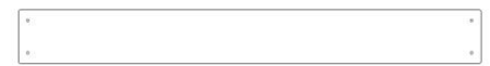
Y1 | PANNEAU MURAL - W4L14616 (x2) | 5/8 po x 4 po x 34 5/8 po (16 x 102 x 880)
