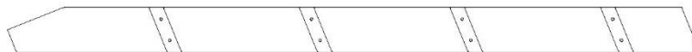
H74 MONTANT GAUCHE - W4L17611 (x1) 1 3/8 po x 3 3/8 po x 50 3/4 po (36 x 86 x 1290)
