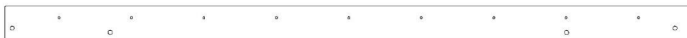
H3 SUPPORT DE PLANCHER - W4L22677 (x1) 1 po x 3 3/8 po x 64 3/4 po (24 x 86 x 1644)
