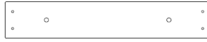
H82 | PANNEAU DE FIXATION - W4L17613 (x1) | 1 po x 3 3/8 po x 19 1/8 po (24 x 86 x 486)
