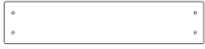
M20 | PANNEAU MURAL - W4L14590 (x2) | 5/8 po x 3 3/8 po x 16 1/4 po (16 x 86 x 412)
