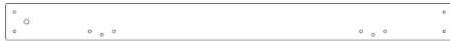
M33 | PANNEAU MURAL - W4L22710 (x1) | 5/8 po x 3 po x 36 1/2 po (16 x 76 x 926)
