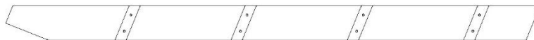
H75 MONTANT DROIT - W4L17612 (x1) 1 3/8 po x 3 3/8 po x 50 3/4 po (36 x 86 x 1290)
