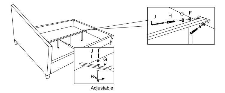
Assembly Iron Pipe(K) to Iron Pipe (O) and Iron Pipe(C) use Bolt(L), Flat Washer(F), Lock Washer (G), Nut(M) by Allen Wrench(J) & Wrench(N).
