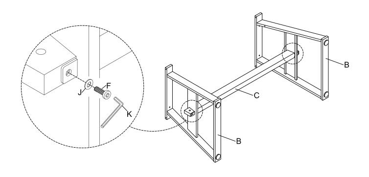
Attach the Support Bar (D) to the Frame (B) using Bolt (F) and Flat Washer (J) with the Allen Key (K).
