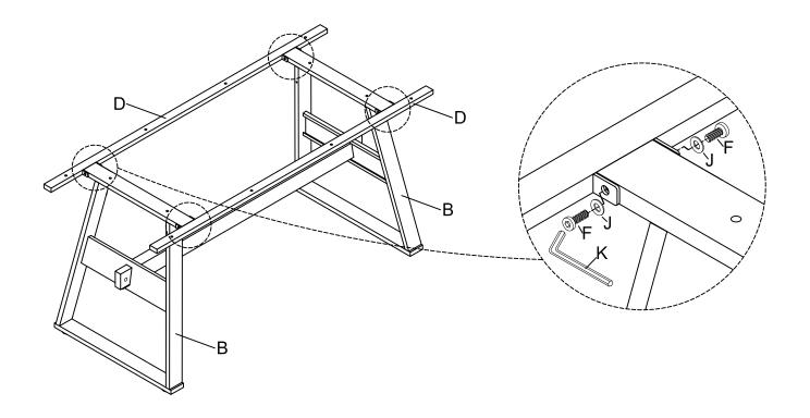
Attach the Frame (B) and the Support Bar (D) to the Top (A) using Bolt (G) and Flat Washer (J) with the Allen Key (K).
