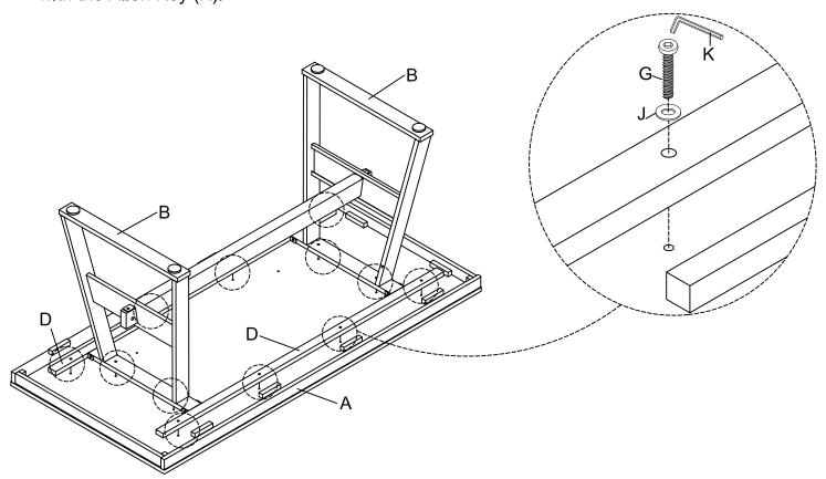
Attach the Support Tube (E) to the Top (A) and the Frame (B) using Bolt (F) and Flat Washer (J) with the Allen Key (K).
