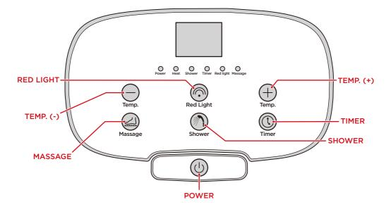
**POWER:** Press to turn machine on and off. When turned on, the machine will automatically begin to heat the water. The power and heat indicator lights will turn on.
