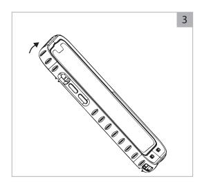
Move the top of the Rugged Phone Case over the top of the iPhone ensuring the case fully covers the iPhone before using the case.
