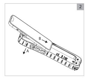
(A) Bend the Rugged Phone Case top down and (B) insert iPhone into the Phone Case inserting the bottom of the phone first then pressing down into the top of the Case.
