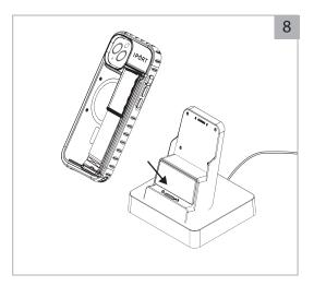
To charge the iPhone in an IPORT Phone Dock or MultiDock place the iPhone with the Screen facing the back of the dock, If not the hand strap will interfere with docking and the iPhone will not charge.
