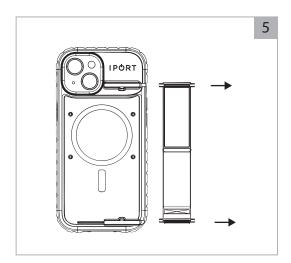
Remove the Strap and replace as needed. To reinstall slide the clips in reverse order as removal.
