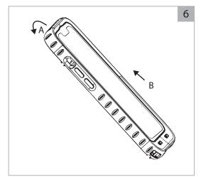
To remove the iPhone (A) first flip the top of the case over the top of the iPhone. (B) Next slide the iPhone towards the top of the **DO NOT** pull the iPhone towards you, slide it up away from the bottom of the case.
