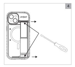
To replace or service the hand strap use a flat head screwdriver and press the small silver trigger under the strap loops, slide each loop towards the outside of the iPhone case.
