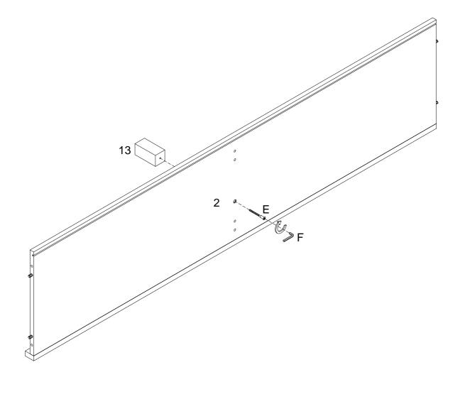
Now, you will attach the Middle Divider Panel (6) to the top of the Bottom Panel (2) using 50mm Screws (E).
