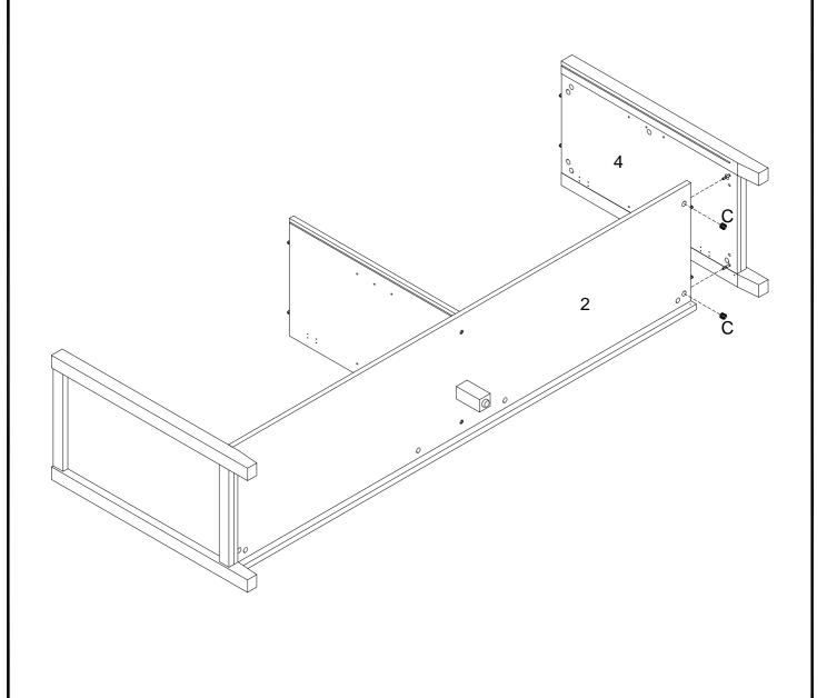
Secure the corners of the Bottom Panel (2) with 15mm Screws (K).
