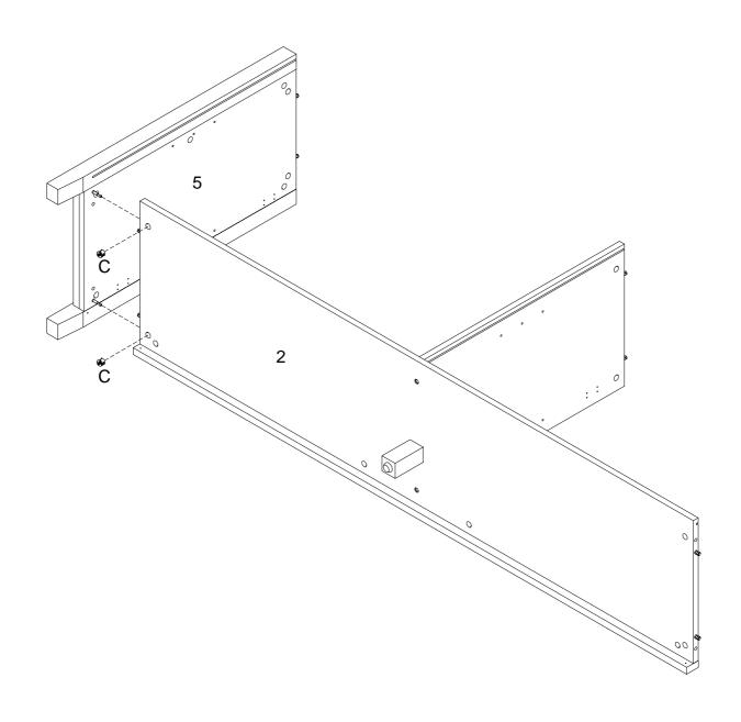
Connect the Left Side Panel (4) to the Bottom Panel (2) and secure with Cam Locks (C).
