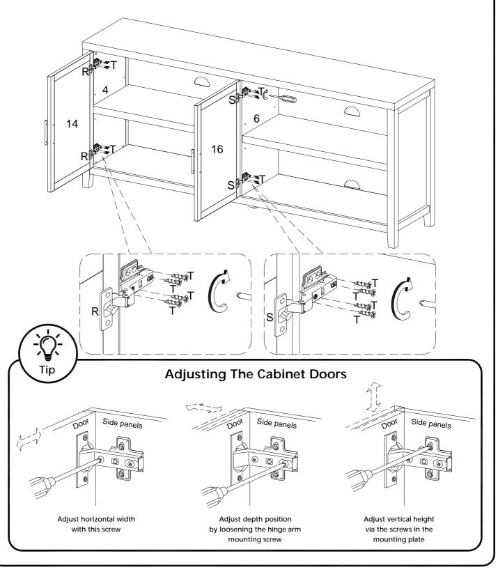
Now, attach the hinges on the Left Center Door (15) and Right Door (17). Use the 13mm Screws (T) to secure.
