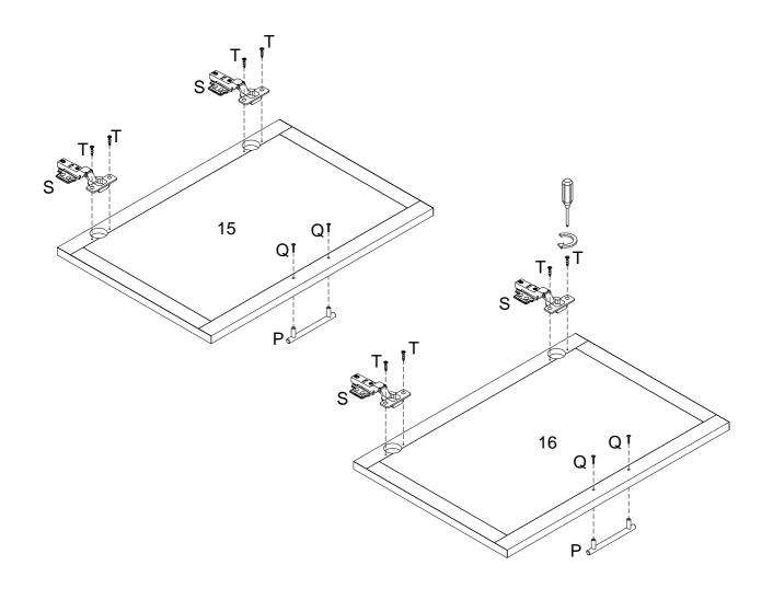
Next, we'll attach the doors. Attach the hinges on the Left Door (14) and the Right Center Door (16) to the sideboard and secure with 13mm Screws (T). Pay careful attention to ensure that each door and hinge is attached to the correct area.
