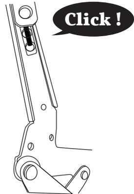
Firmly push each side into place one at a time. **You should hear a click** when the chair back locks into place on each side.
