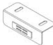
A2 SUPPORT MAGNÉTIQUE- A4M03028 (x1) 1"x1 1/4"x3 1/8" (25x31x80)
