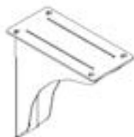
A12 SUPPORT DE TABLE BAR - A4M03022 (x2) 3 3/4"x7 7/8"x8 7/8" (95x200x225)
