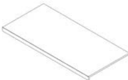
M1 ARMOIRE D'ANGLE EN MARBRE- A4M03035 (x1) 1 15/16"x24 13/16"x51 7/8" (50x630x1317)
