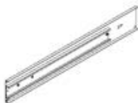
A10 MONTAGE DU SUPPORT DE GLISSIÈRE - A4M03083 (x6) 15/16"x3 3/8"x22 5/8" (23x85x575)
