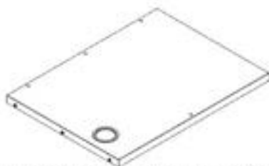
T6 ASSEMBLAGE DE PLATEAU DE FOUR - A4M03070 (x1) 1 3/8"x23 3/8"x31 7/16" (35x594x798)
