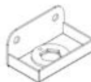
A9 SUPPORT DU TUYAU D'ARROSAGE - A4M03060 (x2) 1 1/4"x1 7/16"x2 9/16" (31.5x36.5x65)
