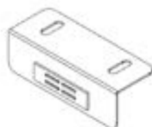
A2 SUPPORT DE MAGNET - A4M03026 (x8) 1"x1 1/4"x3 1/8" (25x31x80)
