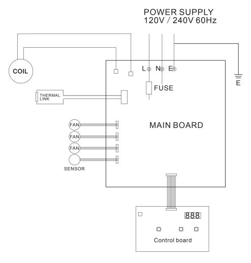
This circuit diagram has been provided to assist qualified electricians; only SPECTRUM™ service agents or qualified electricians should carry out repairs if required.
