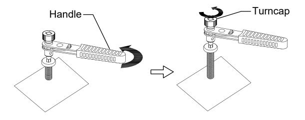
Attach Rail Support Bar (D) to Rail Sections (A) & (C), insert the Bolt (K), turn the Ratchet Tool (P) to tighten them. Attach Rail Support Bar (D) to Rail Sections (B) & (C), insert the Bolt (K), turn the Ratchet Tool (P) to
