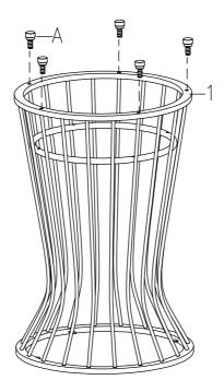
Put Glass Pads (B) onto Metal Base (1) before putting the Glass Top (2) as shown below.
