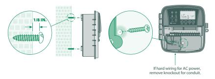
For installation in drywall, use drywall anchors (included in package).
