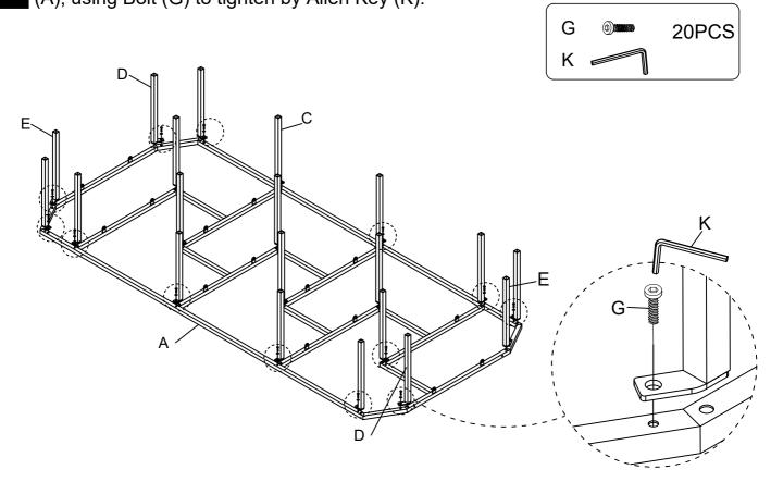
Assembled Back Panel (B) to the assembled Support Tube (C), Support Tube (D) & Support Tube (E), using Bolt (H), to tighten by Allen Key (K). Attach one metal panel of Anti-Tipping Kit (M) to Back Panel (B) using Bolt (H) by Allen Key (K).
