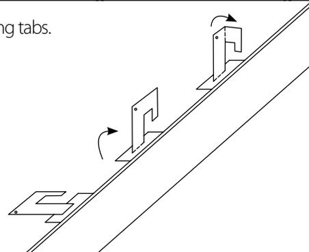
4 Place fixture into the T-grid ceiling panel. Secure to structure and/or grid per state and local codes.
