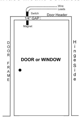
Attach switch to header or side of door or window frame (NOT on hinge side)
