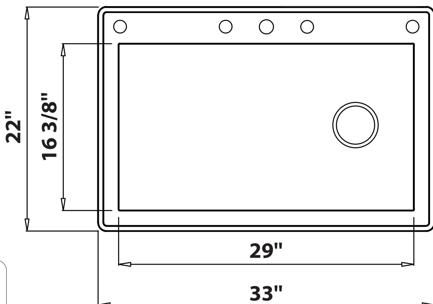
NOTE: Cutout template is provided as a guide ONLY and must be checked against actual sink to verify correct fit.
