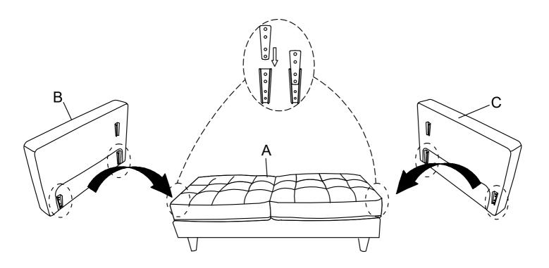
3 Hook on the Back Rest (D) to the Left Arm (B) & Right Arm (C) properly.
