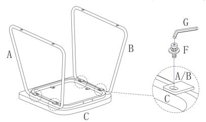
Take the Allen Key, and turn the bolts until the legs are secure. DO NOT TIGHTEN COMPLETELY. Stop when you feel you are adding force to tighten the bolt.
