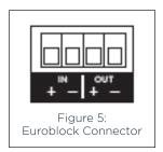
Strip approximately .1875" (5mm) of the insulation off each wire. Insert the wire into the correct square opening on the connector. Use a small flat head screwdriver to tighten the corresponding screw to secure the wire (see Figure 6).
