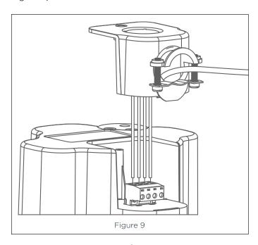
The included conduit clamp/wire strain relief can be installed on the top or the side of the terminal cover using either available knockout. Once the clamp is installed, route the wires through the strain relief fitting. Tighten the screws on the clamp to secure the conduit/wires the wires. Make sure not to over-tighten the screws and damage the wire.
