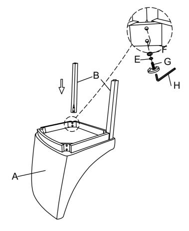
Take the Allen Key, and turn the bolts until the legs are secure. DO NOT TIGHTEN COMPLETELY. Stop when you feel you are adding force to tighten the bolt. 2 Then attach the Left Back Leg (C) & Right Back Leg (D) to the Chair Body (A) using Bolt (G), Lock Washer (E), Flat Washer (F) in both holes of Left Back Leg (C) & Right Back Leg (D) and Chair Body (A). Turn the Allen Key (H) in Bolt (G).
