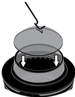
After a Wood Pack or firewood has been added, place the top piece back on with the poker. Ensure that it is securely nested.
