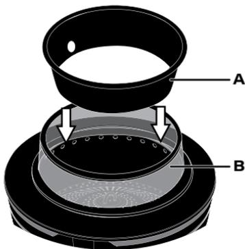
Set the lower screen (B) on the top ring of the Fire Pit. Place the heat deflector (A) inside the lower screen.
