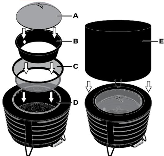
When the Fire Pit is not in use, you may nest the accessories inside Fire Pit. First, invert the lower screen (C) and place it inside the Fire Pit (D). Next, put the heat deflector (B) right-side up in the inverted lower screen (C). Place the upper screen (A) on top. Finally, place the cover (E) (included with the Fire Pit purchase), over the top.
