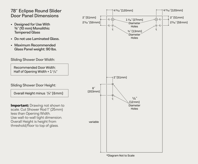
If fabricating custom glass for the Eclipse Round Slider Shower Hardware Kit, please use the specs below for the Fixed Panel if your opening is under 531/4" in width.
