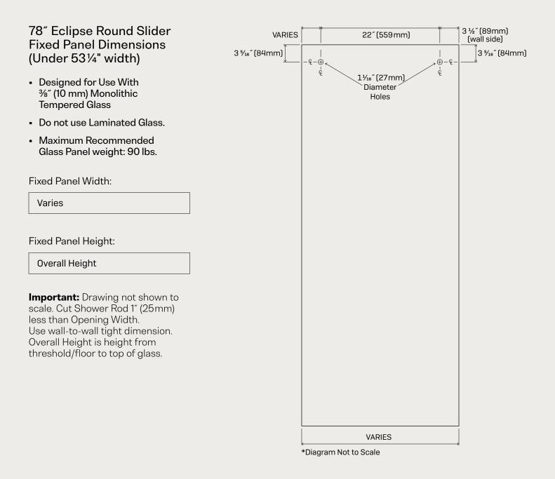
If fabricating custom glass for the Eclipse Round Slider Shower Hardware Kit, please use the specs below for the Fixed Panel if your opening is over 531/4" in width.
