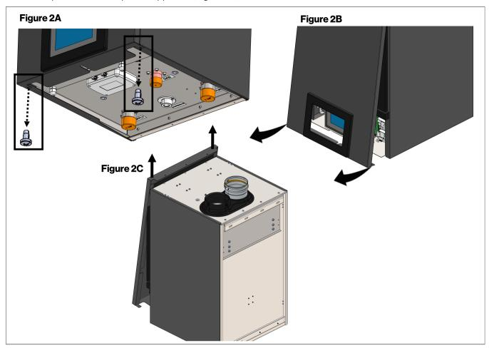
5. Use a Phillips head screw driver to remove three screws holding left side panel (Figure 3A). Rotate the side panel out (Figure 3B), push the panel up to clear the cutout located on back side of boiler, and pull the side panel out (Figure 3C).
