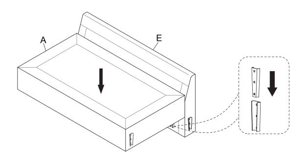
4 Hook the Seat Frame (A) & Backrest (E) onto the Arm (C) properly.
