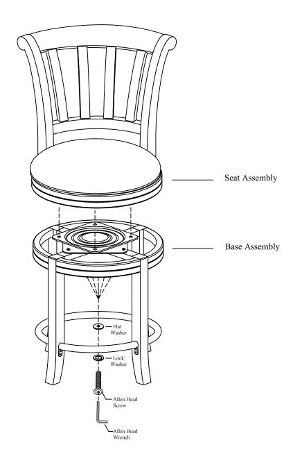
Attach the Seat Assembly to the Base Assembly with hardware as shown.
