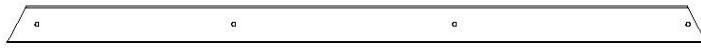
M3 | RAIL ANGULAIRE AU SOL - W4L13217 (1) | 5/8 po x 3 3/8 po x 65 5/8 po (16x86x1666)
