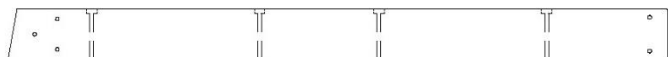
SB74 | POUTRE DE BALANÇOIRE 2 POSITIONS - W4L13291 (1) | 2 po x 5 1/4 po x 68 3/4 po (50x134x1745)
