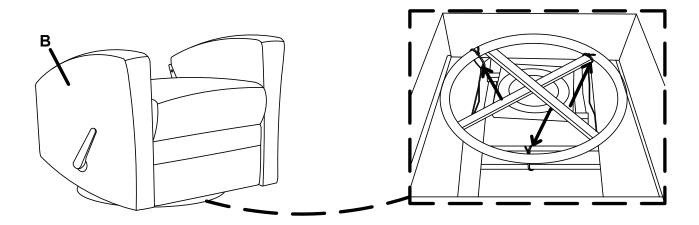
Align the female brackets at the Back Rest (A) onto the male brackets at the Seat (B), insert to the end, and make sure the brackets are secured in position.
