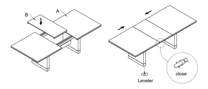
Pulling out and opening the Table Top (A) can storage the Table Leaf (B) inside the table.
