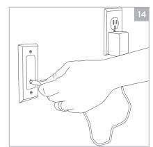
Plug power adapter into electrical receptical and plug power adapter DC plug into wall plate. Only use a LAUNCH power supply with a LAUNCH system.
