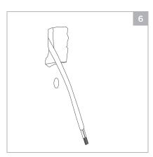
Receive wire through wall plate cutout. \*NOTE: For help going through a fire block refer to: iportproducts.com
