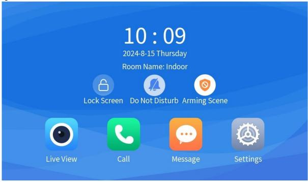
The home screen displays the current time (set on the Web), and supports Lock Screen Manually, Do Not Disturb, Arming, Live View, Make Calls, Answer Calls, Message, and Settings.
