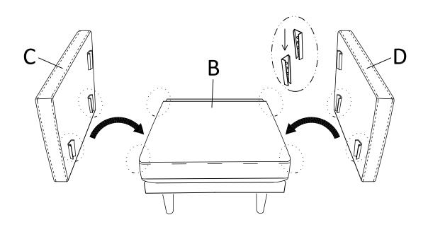
Hook on the Back Frame(A) to the Left Panel(C) & Right Panel(D) properly.
