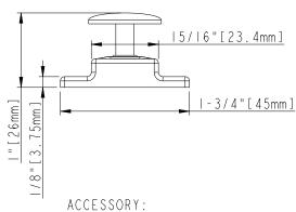
SCREW:8-32XI" 2PCS BREAK AWAY SCREW:8-32x45 2PCS ALL SCREW MATERIAL: STEEL-SAE1006
