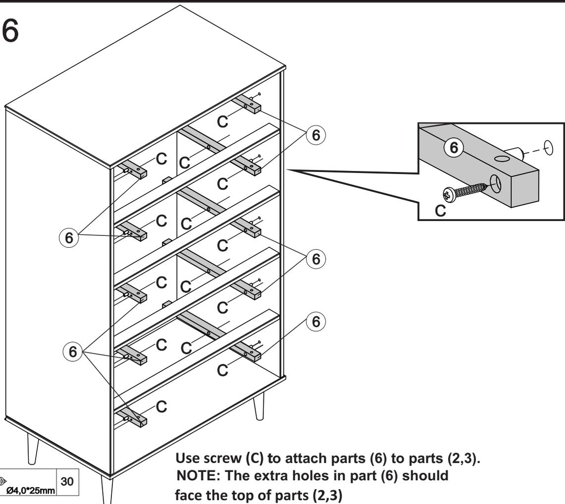
Use screw (C) to attach parts (6) to parts (2,3).
