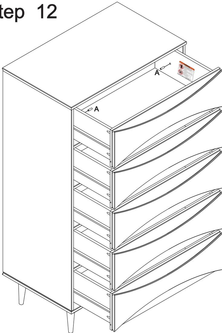
Insert wood dowel (A) on the inside of all drawers while drawer is inside the unit. Make sure dowel is flush with panel.
