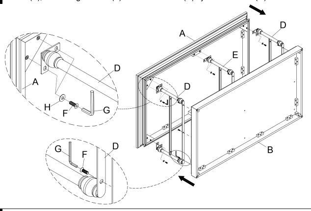
Assembly the Shelf (C) onto the Side Frame (D) and Middle Frame (E) then using the Bolt (F) by Allen Wrench (G).
