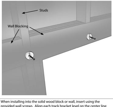
provided wall screws. Align each track bracket level on the center line mark and install with (5) bracket screws.
