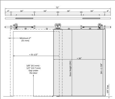
When installing into drywall, a piece of solid wood blocking is required to be mounted inside or outside of the wall before proceeding with the track installation. Position the solid wood blocking with track by measuring up from the door height (DH) + 1-7/8'' to the center of the track. This allows a 3/8" - 1/2" gap at the bottom. For outside wall blocking, ensure it is level and leave a minimum of 2" from the end of the blocking to the side of the opening.
