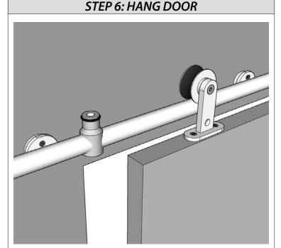
Place the assembled door onto the mounted track. Ensure all parts are functioning correctly by sliding the door side-to-side.
