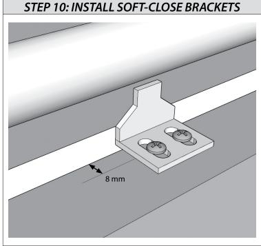
After door stops are adjusted, measure and mark 8 mm from the back on top of the door. Position the Soft-close Brackets to engage the Softclose guide when it opens and closes. Mount and adjust the Soft-close Brackets using the screws provided.
