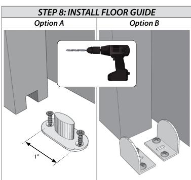
Once the door is plumb, position the floor-mounted door guide inside the mortised door for Option A, or outside the door for Option B. Line up the guide close to the opening. Slide the door side-to-side to ensure functionality for final placement then mark holes with a pencil and predrll 1/4" holes. If drilling directly into concrete floor, use the provided anchors.
