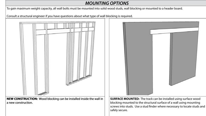
Typical solid wood surface blocking should be 73" (L) x 5-1/2" (H) x 7/8" (D) for the 72" length track.
