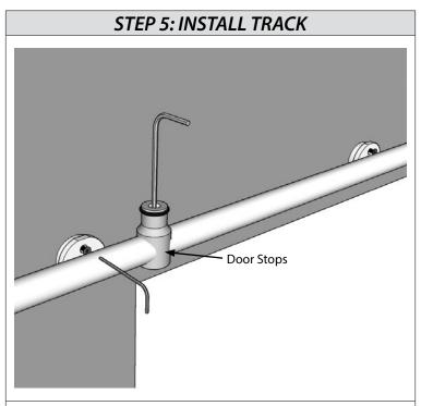
Determine where your Door Stops needs to be placed prior to mounting. Insert one Door Stop on each side of the track inside the first mounting hole before securing if needed.
