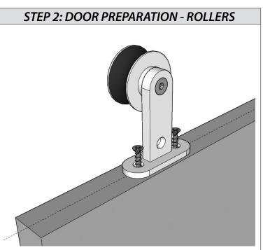
Determine your Door Roller Hardware position. Measure and mark the center line on top of the door. Position each roller on top of the door a minimum of 2" from the edge or center of the stile. Install with (4) Door Roller Hardware Screws.
