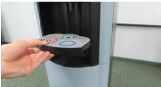
2. Depress the clip visible through the slot in the alcove and lean the top of the door forward
