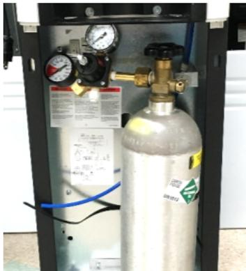
5. Connect CO2 blue tube to the quick-fit connector on the CO2 pressure regulator
