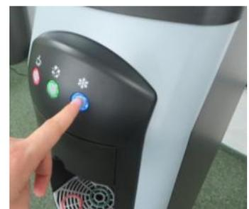
4. Draw water from the hot faucet. To do so press and hold hot water button (marked with RED light) until red light begins to flash, release the button to unlock and press it again. Keep the button pressed until water flows freely and all air is expelled (filling hot tank with water will take no more than 2 minutes)
