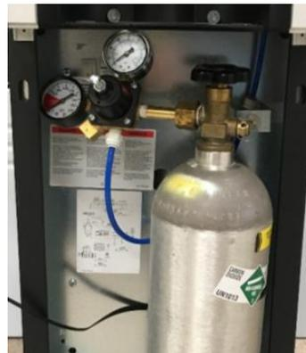
6. Place the cylinder in the compartment and secure it with the Cable Tie
