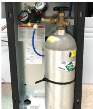
9. Set the gauge on the OASIS supplied pressure regulator to 60 psi
