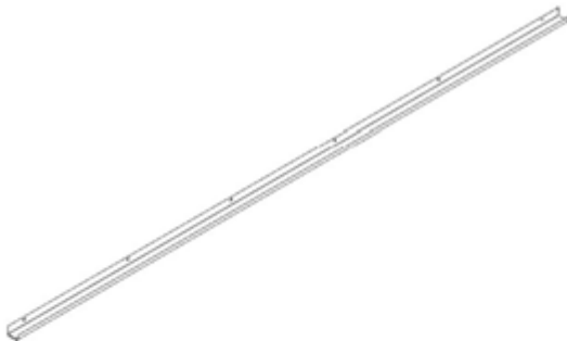
G01 GUTTER - A4M01993 (x2) 1 9/16"x1 15/16"x108 7/8" (40x50x2765)
