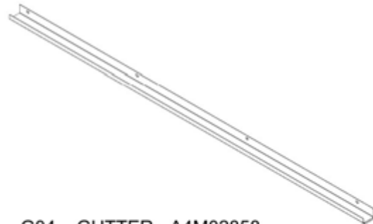
G04 GUTTER - A4M02858 (x2) 1 9/16"x1 15/16"x65 15/16" (40x50x1675)
