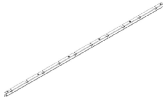
M01 LOUVER MOUNT - A4M02864 (x2) 1"x1 15/16"x65 7/8" (25x49x1673)
