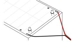
2. Pull tab off the bottom side of Rubber Bumper. Place Rubber Bumper on the top side of the Flex Sheet and press down to secure.
