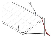
1. Use screws with the pre-cut mounting holes to secure the Flex Sheet Light to the installation surface. Nylon washers can be used for a more secure installation.
