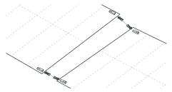
2. To connect additional Flex Sheets, firmly push one end of the connector pins into the push connectors on the end of one sheet, then push the other end into the connectors on the end of the next sheet.
