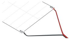
1. Make sure connection wire from the power supply is stripped 1/4". Insert wire into push connectors on the Flex Sheet, red wire to positive (24+) and black wire to negative (24-).
