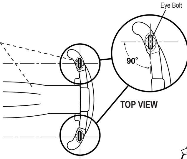
It is helpful to use a screwdriver to hold eye bolt in place when tightening lock nut.
