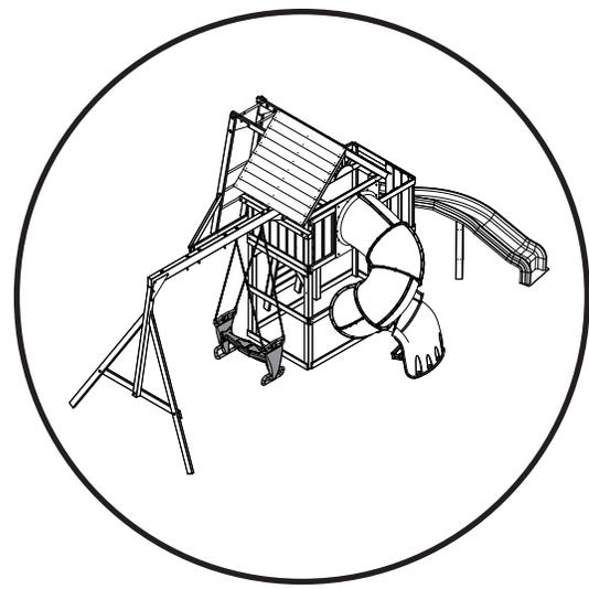
Eye bolts should be oriented perpendicular with Glider seat.
