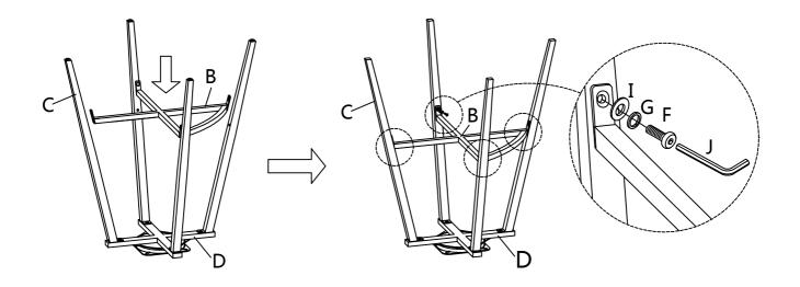
Stand the metal base up. Use Long Bolt (E), Spring Washer (G), Flat Washer (H) with Allen Key (J) to fix Rotary Turntable (D) and Leg (C).
