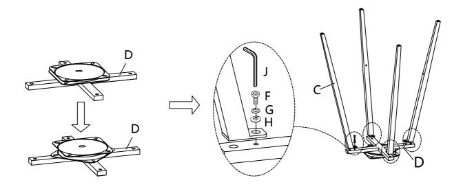
Put Leg Support (B) between assembled leg frame. Use Bolt (F), Spring Washer (G), Flat Washer (I) with Allen Key (J) to fix Leg Support (B) and Leg (C).
