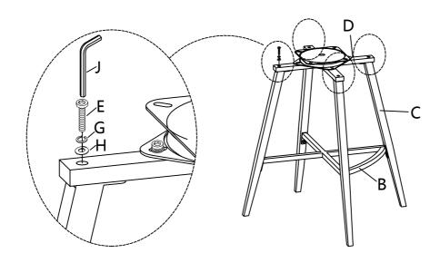
Attach Rotary Turntable (D) to the bottom of Chair Seat (A) using Long Bolt (E), Spring Washer (G), Flat Washer (H) with Allen Key (J).
