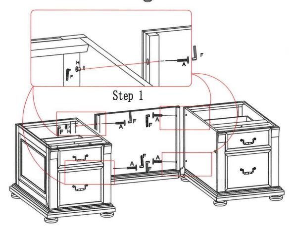
Step 1: Assemble the left and right bases and the center panel with Bolt (A) (H), Lock Washer (B) and Washer (C) using wrench (F)
