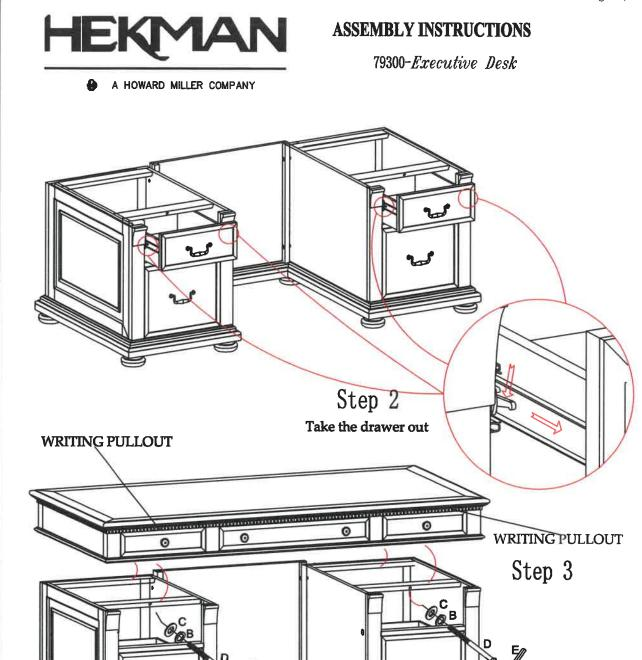
Step 2: Remove the upper drawers in both pedestals - Open drawer fully to expose the release levers in the center of the drawer slide. Push the lever on the left side up, and the lever on the right side down to release drawer. With levers pushed gently tug the drawer out of the desk
